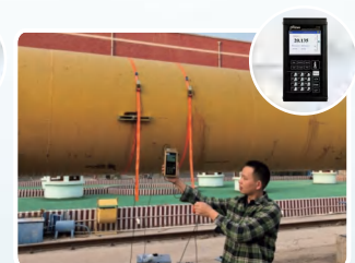
Measurement on a 1.8m Pipeline
